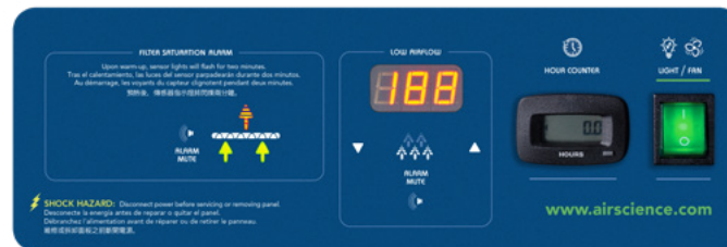
FSA/Autocal Control Panel
